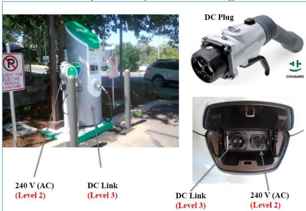
Figure 1. AC and DC charging units (Kintner, 2013)
