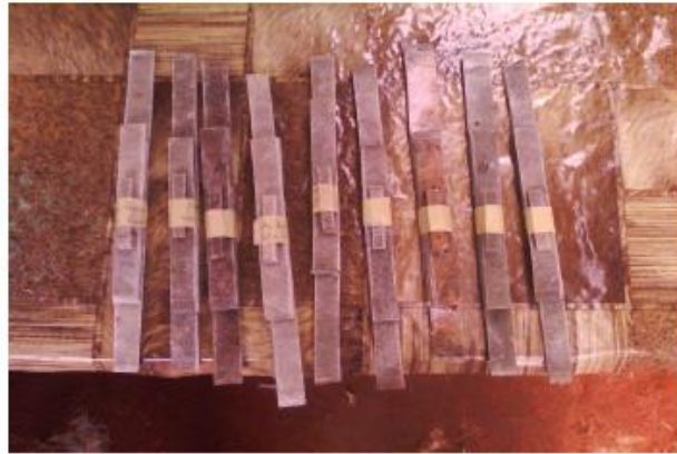
Figure 2. The fabricated epoxy resin composites samples produced from the natural Coir fibre.
