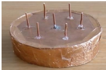
Figure 7. the proposed prototyped 7 element ESPAR antenna
