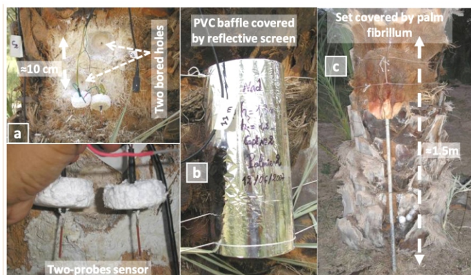
Picture 3. Details of the TDP Sap flow sensor installation on the date palm trunk with adopted insulation precautions (Photos taken by I. BEN AISSA)
