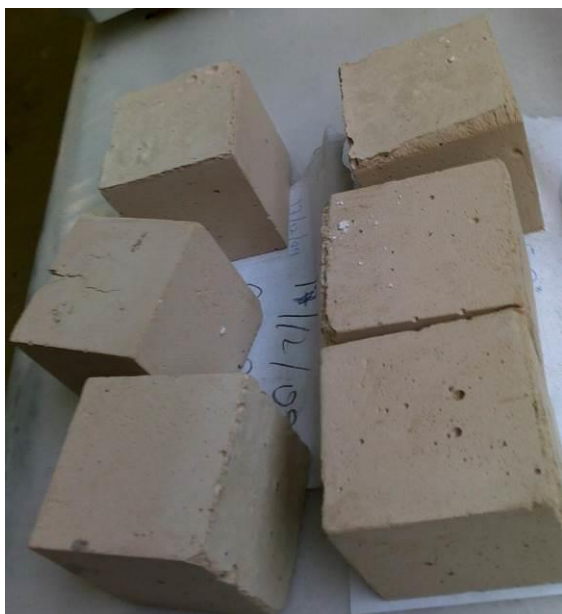
Figure 3. Hardened marble cement composites after elevated temperature
