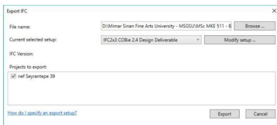
Figure 15: Revit IFC2x3 COBie 2.4 Design Deliverable View Exporter
