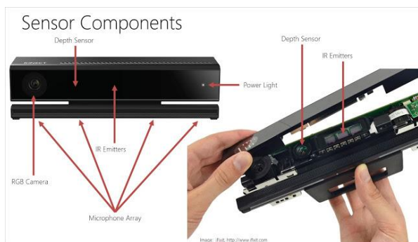
Figure 1. MS Kinect V2 and its components [1]
