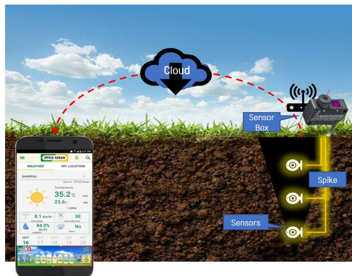
Figure 2. Control of soil condition via smart phone and sensors.
