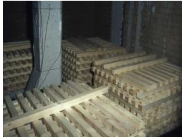
Figure 1.1: Concrete column in test furnace of SFB with wood cribs as fire loads
