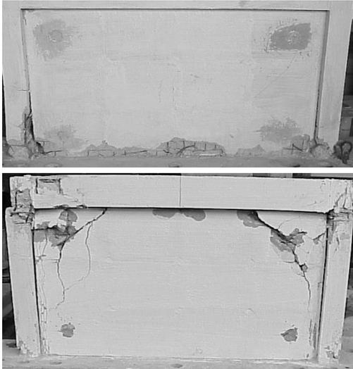
Fig.9. Photographs of first storey infills (CI Specimens)
