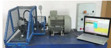
Fig. 1. Brake lining test device used in this study
