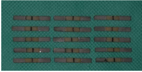
Fig 2. Laser sintered test specimens ready for 3-point-bending test.
