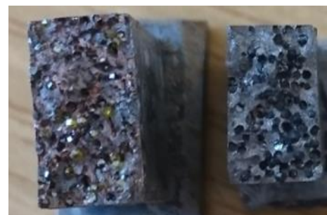
Figure 7. Changing of diamond color at sintering temperature of 1000 °C. Type B segment (on the left) and type A segment (on the right)
