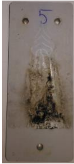
Figure 11. Tracking Formation on Silicon Sample Surface Under the Influence of Electric Field and Magnetic Field
