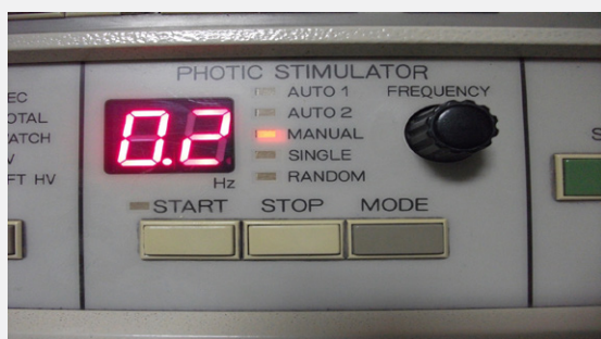
Fig. 2. All frequencies can be manually adjusted and managed by the control button over the EEG device.
