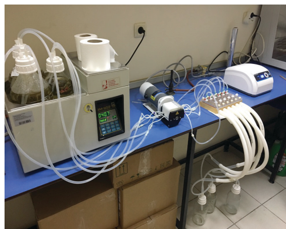
Figure 1. Drip flow reactor used in the study
