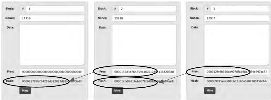
Figure 6: Screenshot from video at https://anders.com/blockchain/ [28.4.2018] with inserted arrows indicating linking blocks through hashcodes
