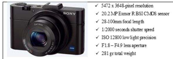
Figure 3. Technical specifications of the Sony RX100II compact camera.
