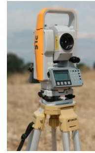
Figure 2. Cygnus topcon ks-102 total-station
