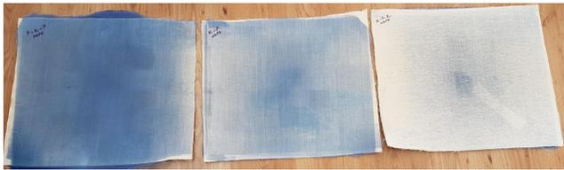
**Figure 1.** H-F-H, H-F and F-H-F composites (left to right)
