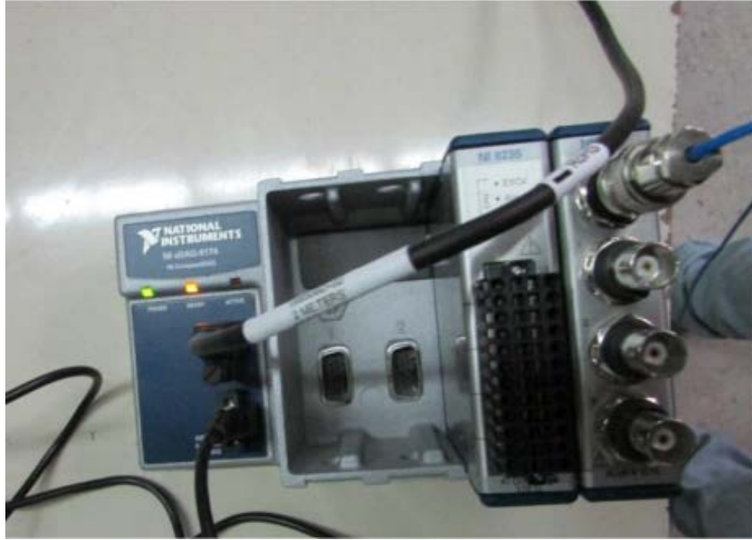
Figure 4. NI 9233-USB-9162 Model Data Collector and Mounting
