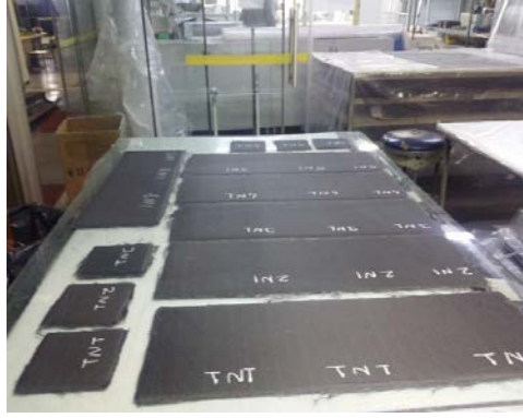
Figure 1. Composite plates after vacuum and curing process
