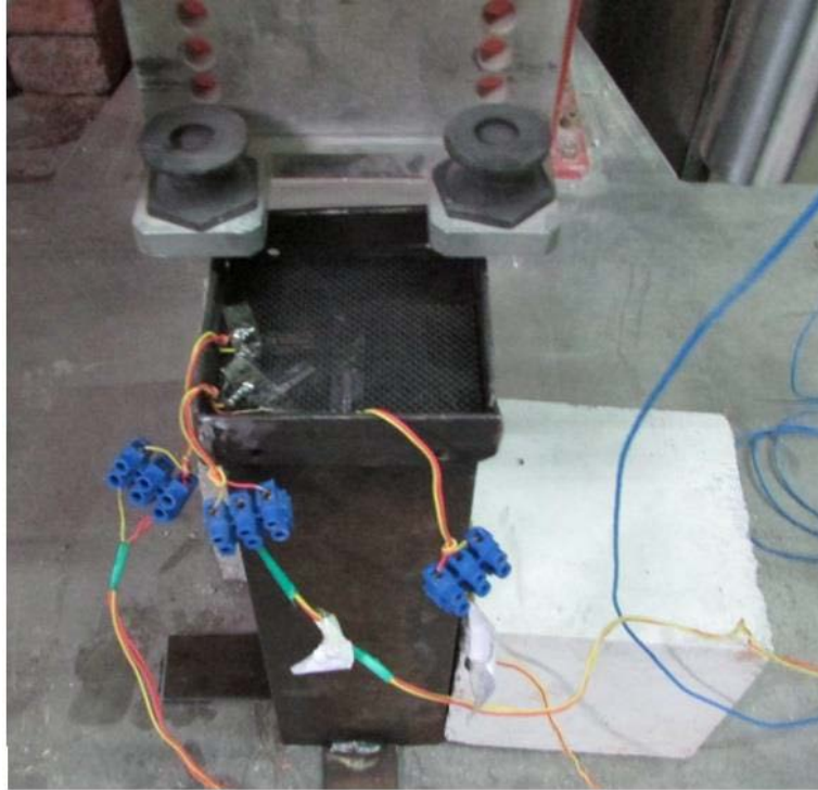
Figure 9. Samples with strain gage
