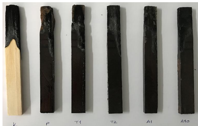
Figure 1. The images of samples after LOI test.
