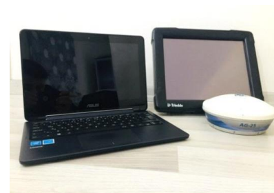
Figure 1. Laptop computer (left), monitor (middle) and GNSS receiver (right) used in the study to record coordinates of the tractor and sprayer
