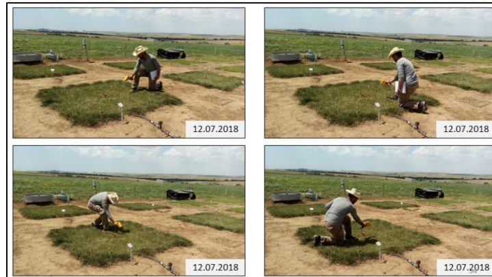
Figure 8. IRTs measurement under a clear sky at four cardinal directions in a plot for sub-treatment (I2:50%) of cool-season turfgrass while determining the NWSB.
