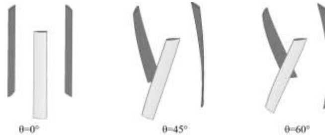
Figure 11. Straight bladed turbine (a), 45° helical turbine (b) and 60° helical turbine (c)
