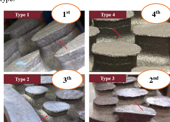
Figure 7. Defect sample on the pillars in 4 types vented discs.
