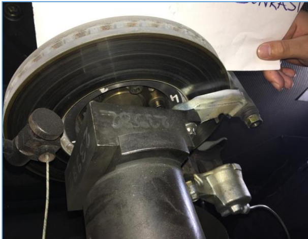
Figure 8. Crack test on bench, mounted rotor on dyno.
