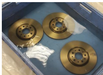
Figure 14. Rotors after crack test with thermal shock.
