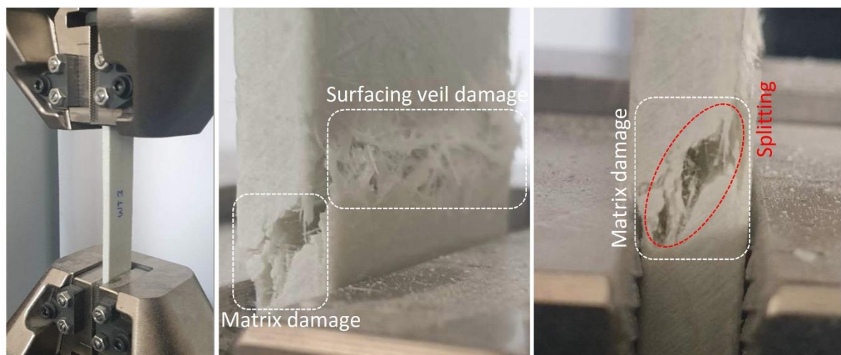
Fig. 7. Tensile test failure in the transverse direction
