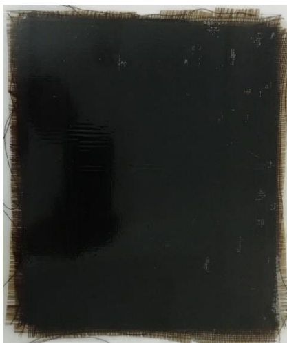
Fig. 2. Basalt/epoxy fiber reinforced composite laminate
