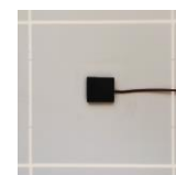
Fig. 2. One of the temperature sensors adhered to the backside of a module
