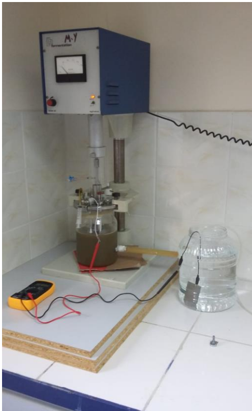
Fig. 3. MFC double system and output voltage measurement
