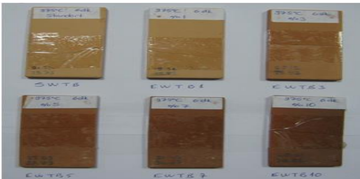
Figure 7. Photographs of EWTB fired at 975 °C and subjected to FBS test.
