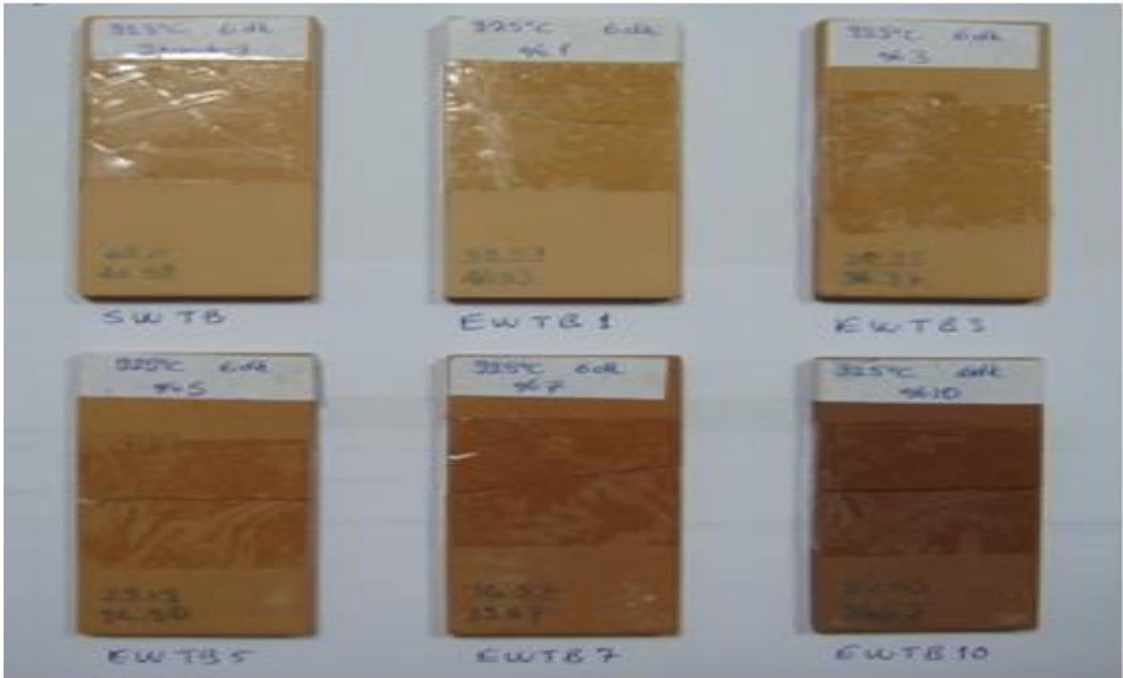
Figure 8. Photographs of EWTB fired at 1025 °C and subjected to FBS test.
