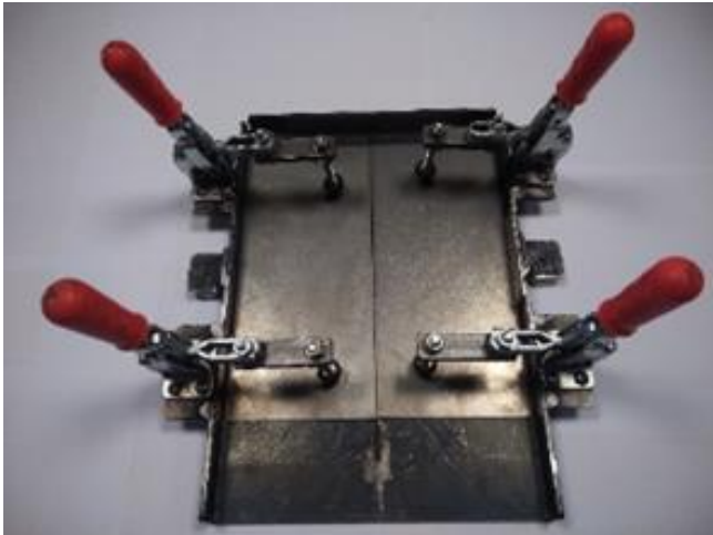
Figure 1. The fixture used in the welding operations
