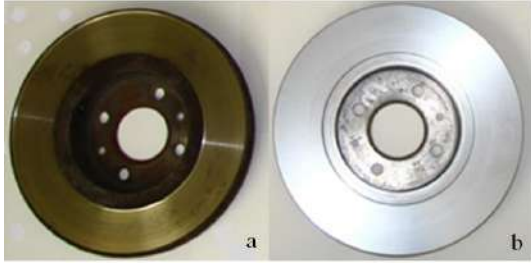
Figure 1. Views of the brake discs used in this study: a-cast iron sample; b-coated sample
