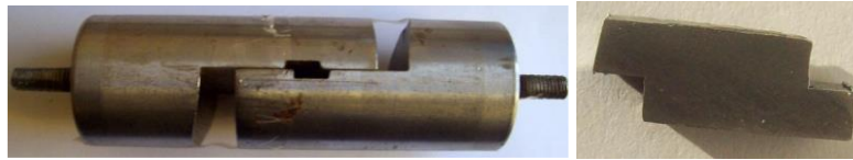
Figure 4. Apparatus for the shear test and the diffusion bonded shear test specimen photo [25]
