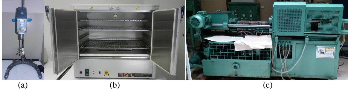
Figure 1. Equipment and machines used in production a) mechanical mixer, b) oven and c) plastic injection machine
