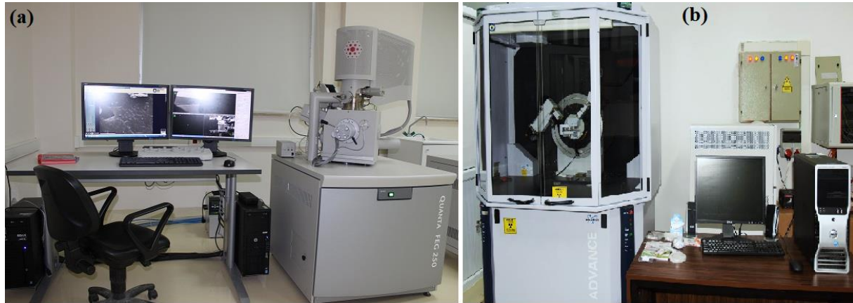
Figure 2. (a) FEI QUANTA 250 FEG SEM analyzer, (b) Bruker D8 Advance XRD analyzer.
