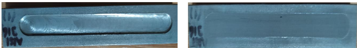
Figure 1: (a) AISI 304 stainless steel substrate, (b) Boron powder laid base
