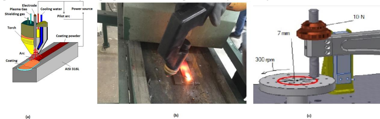
Figure 2: (a)Schematic figure of PTA source and coating process [23] , (b) Sample processed with coating, (c) Wear device schematic picture
