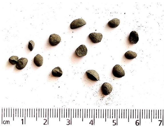
Figure 3. A photographic view of the typical artificial lightweight fine aggregate particles after crushing
