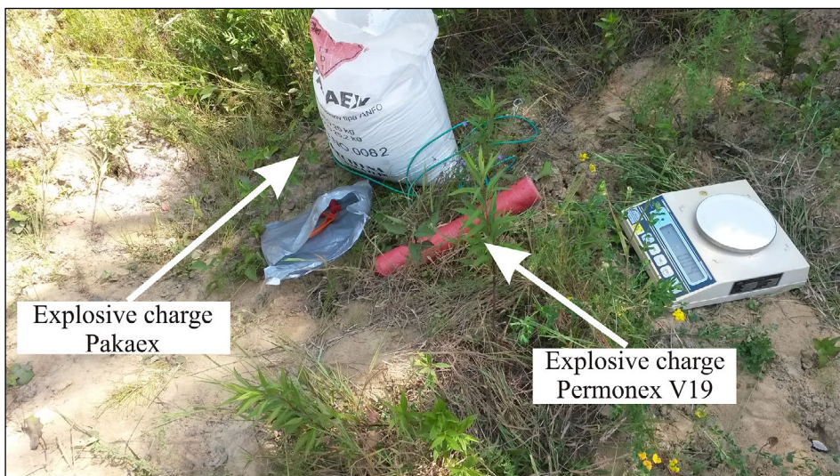
Figure 9- Explosive charge, Permonex V19 and Pakaex (Težak, 2018).
