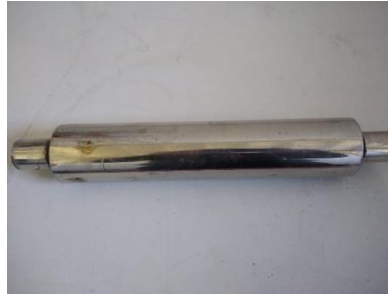
Figure A. Magnetic pipe used for magnetizing water
