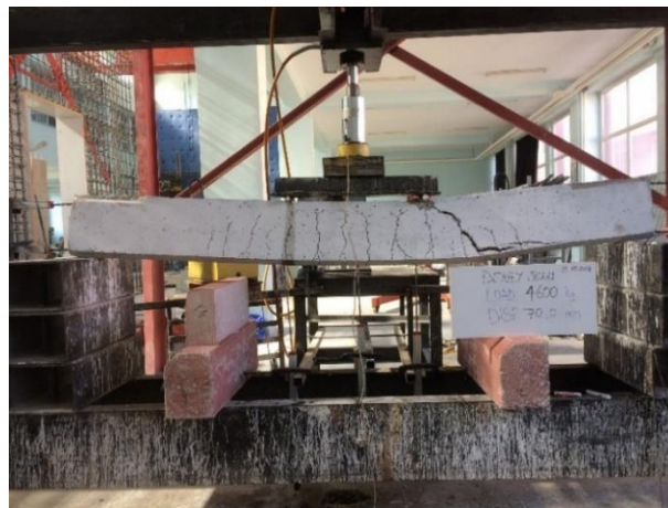
Figure 4. Fractures in specimen (B-1)
