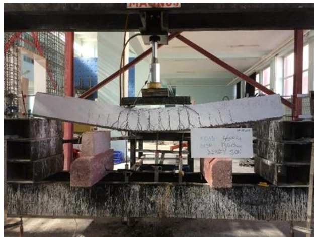
Figure 11. Fractures in specimen (B-7)
