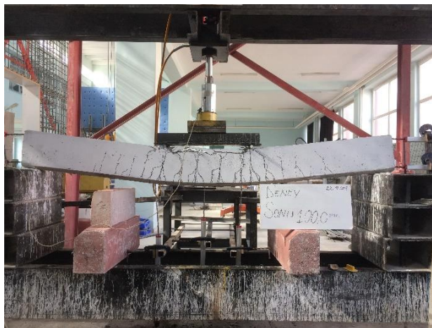
Figure 14. Fractures in specimen (B-8)
