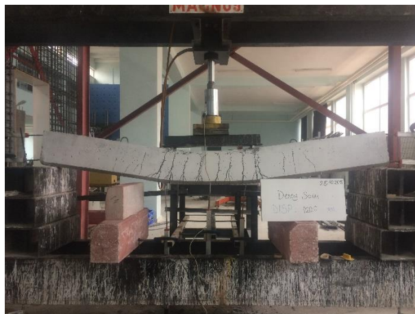
Figure 8. Fractures in specimen (B-6)
