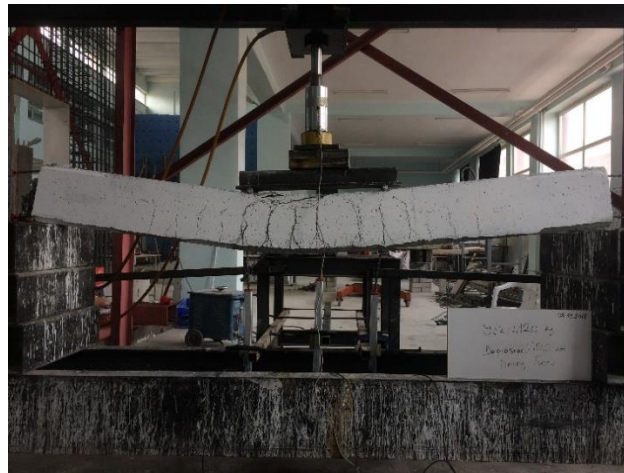
Figure 10. Fractures in specimen (B-3)
