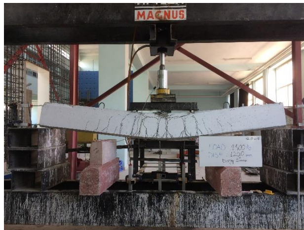
Figure 13. Fractures in specimen (B-4)
