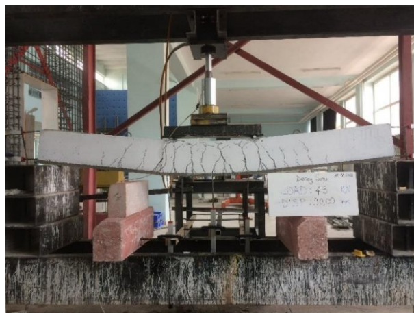
Figure 5. Fractures in specimen (B-5)
