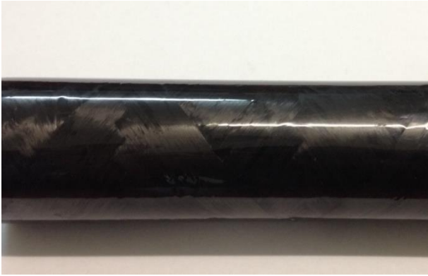
Figure 8. Carbon fiber with 45° after post processing.
