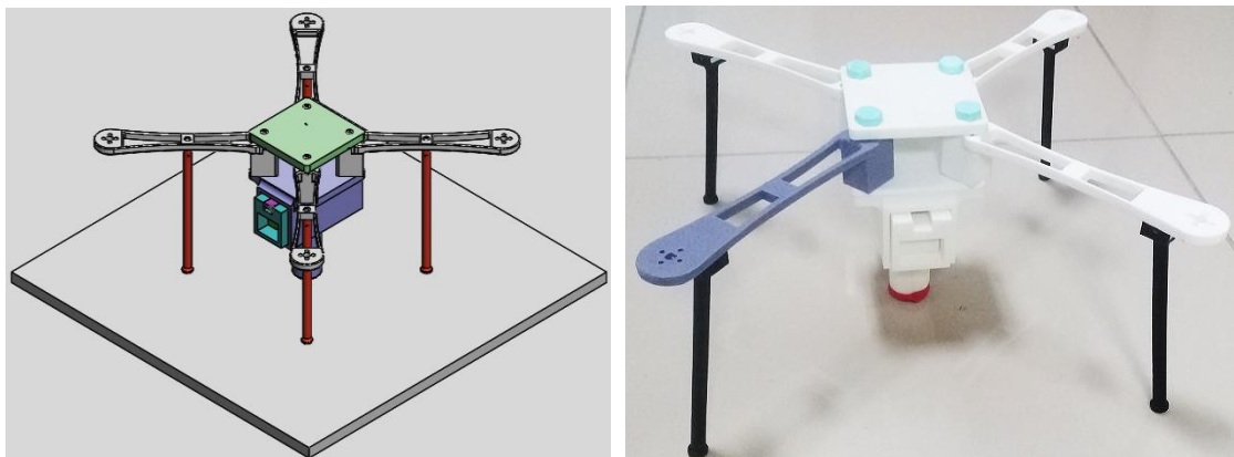
Figure 1. a) 3D model of quadcopter chassis b) 3D printed quadcopter chassis produced from PLA.
