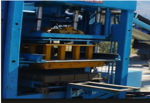
Figure 2. Concrete locked parquet stone production
