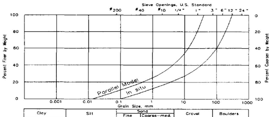
Figure 1: Parallel method illustrated with gradational analysis (Innacchione, 2000)
