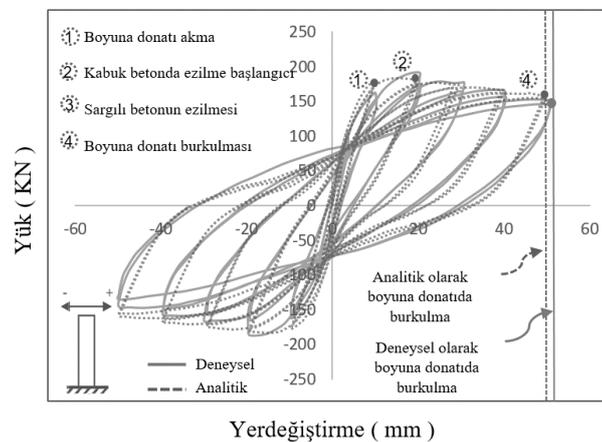
**Figure 3.6:** Experimental and analytical load displacement relationships (Ang vd., 1981.No.3) for a column sample in the experimental database
