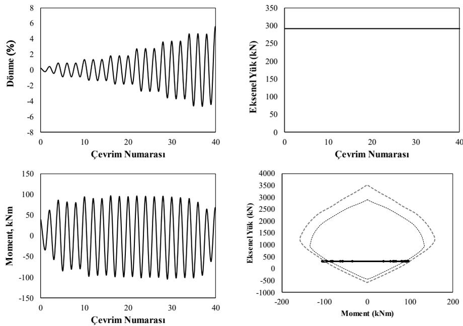
**Figure 3.3:** (a) the demand for rotation in the displacement controlled cyclical loading, (b) the axial loading, (c) the bending moment demand in the cyclic load, (d) the representation of the experimental results on the analytical N-M interaction diagram, on the test sample.
