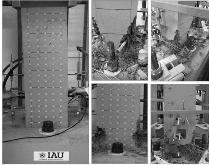
**Figure 3.4:** Photographs of the collapsed test sample during and at the end of the loading
