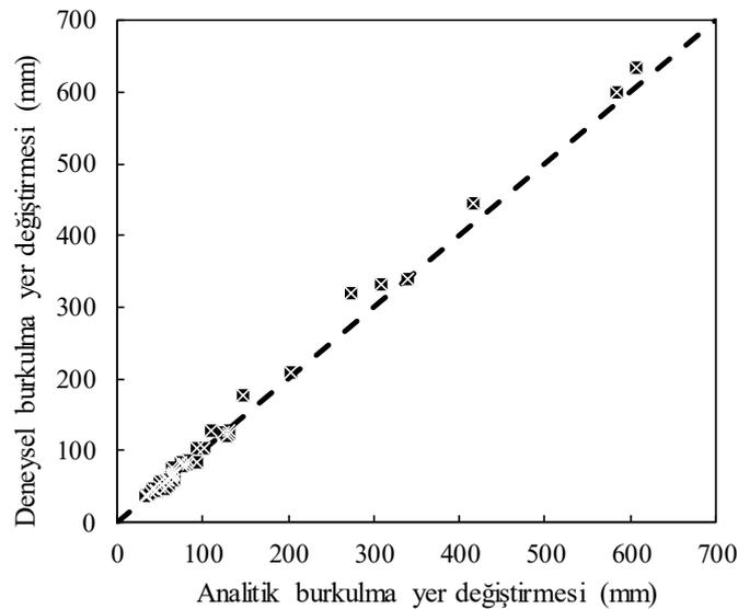
**Figure 3.7:** Comparison of analytical and experimental buckling displacements of column samples in experimental database
