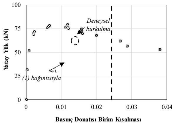
**Figure 3.5:** Comparison of experimental load-pressure reinforcement unit deformation request and analytical buckling deformation limit with experimental results
