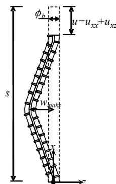
Figure 2.1: Displacement profile of the buckled rebar [10]
