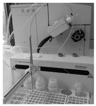
Figure 1. ICP-MS device
