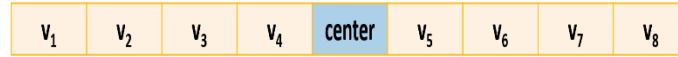
Figure 2. Demonstration of the used 9 sized overlapping block. In the 1D-LBP, the 5th value is assigned as center value, and bits are extracted using center value and other values together
