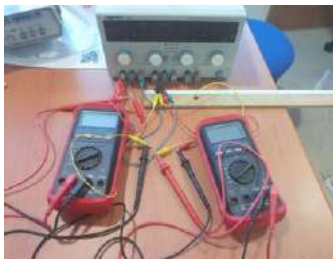
Figure 2. Electrical Conductivity Measurement Setup
