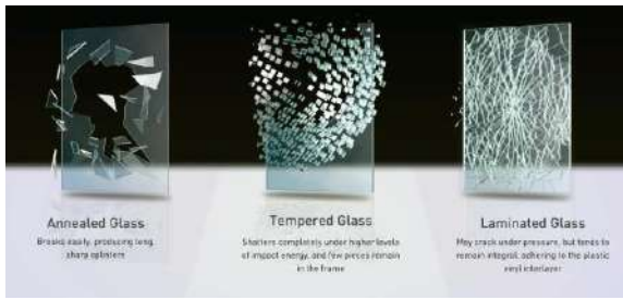
Figure 9. Breaking behavior of annealed, tempered, and laminated glasses [16]
