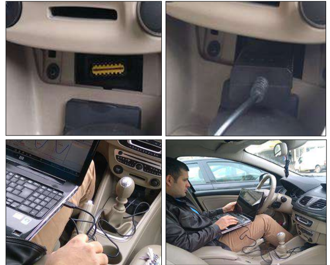
Figure 10. Data acquisition via OBDII
