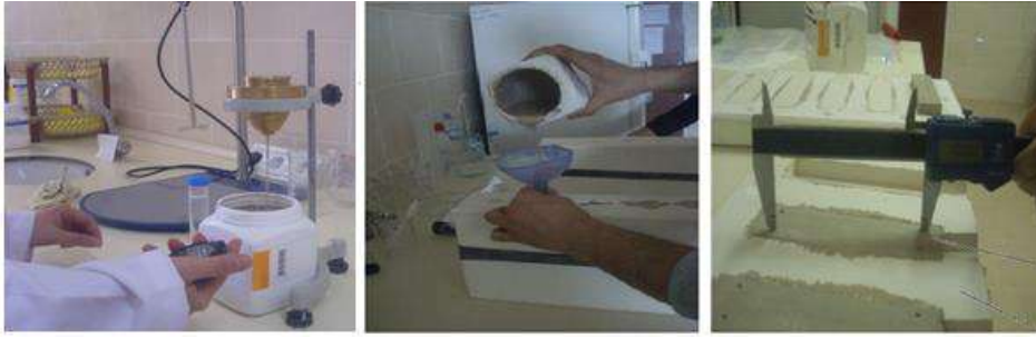
Figure 4 (a) Flow Test of the Slurry with a Ford Cup (b) Slip Casting of the Slurry (c) Measuring the Dimensions of the Bar Shaped Sample after Casting
