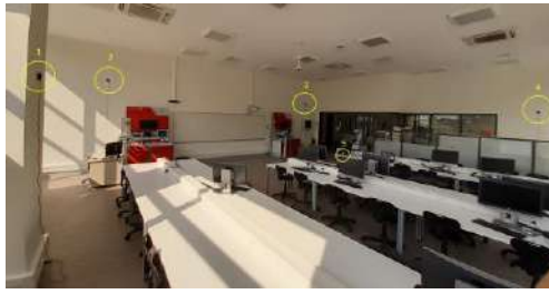
Fig. 8. UWB anchors and the real test environments.
