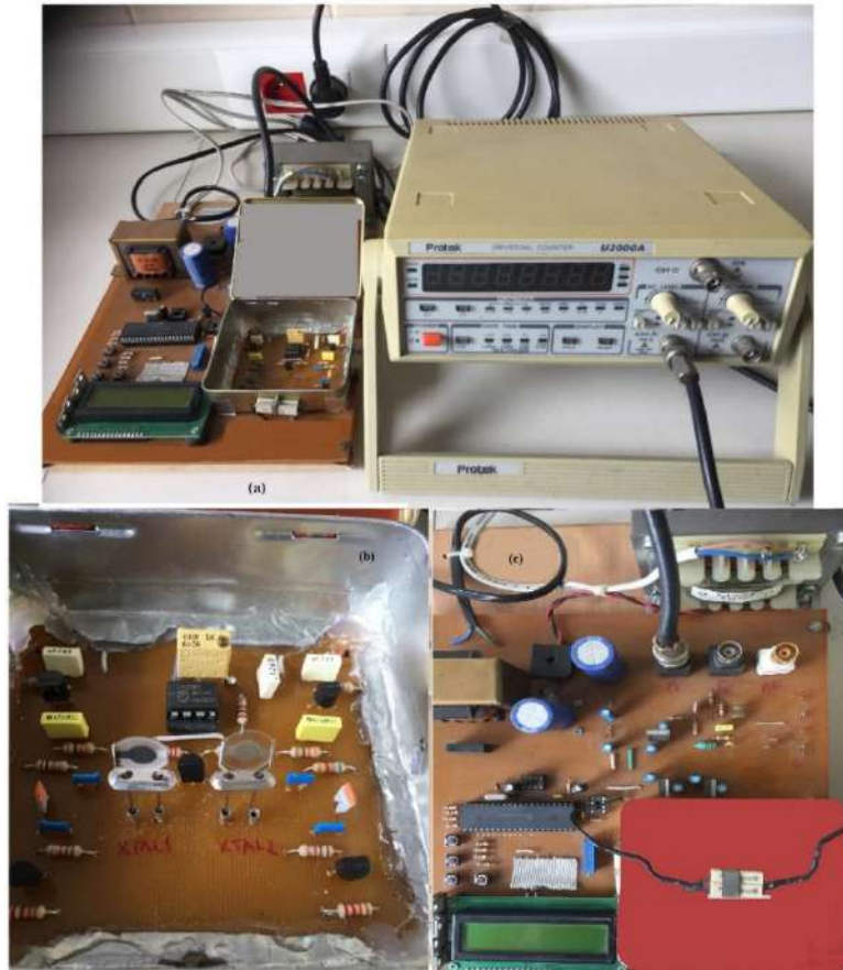
Figure 2. QCM system a) general view of system with frequency counter on right, b) mounted silver electrode quartz crystals, c) temperature controller on crystal mounted chamber (red).
