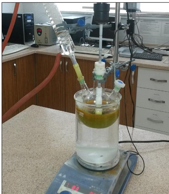
Figure 1- Glass reactor used in the leaching experiments.
