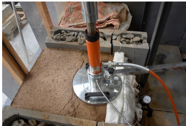
Figure 7. Failure cracks of reinforced earth wall with clay backfill
