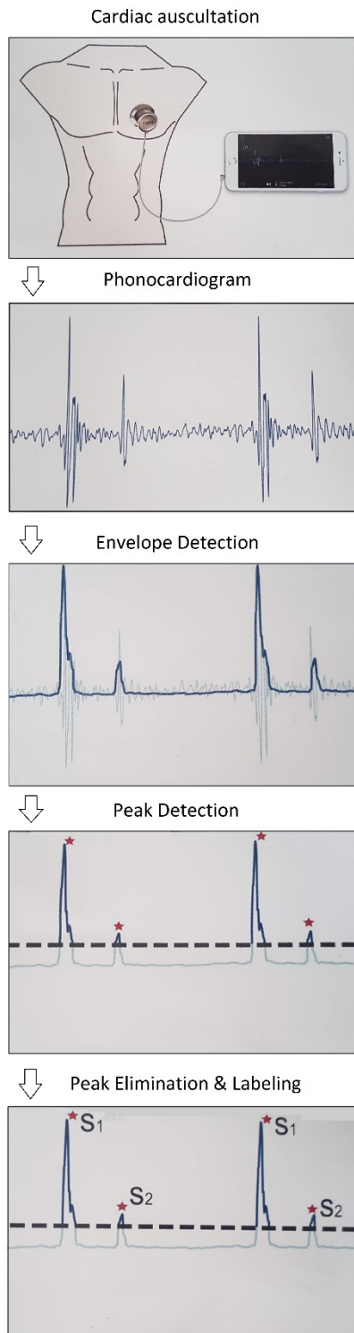
Figure 2 Steps of extracting S1 and S2 heart sound from raw audio data
