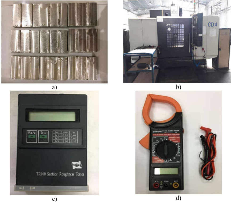
Figure 1. Test setup. a) Experiment samples, b) CNC vertical machining center, c) Surface roughness tester d) Clamp meter
