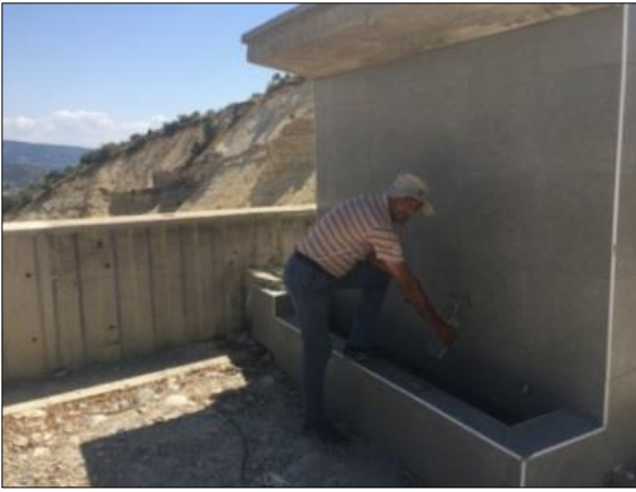
Figure 6. A view of water sampling procedure from cold water fountains (pure and clean natural flowing waters) in the study area by using scaled polyethylene bottles
