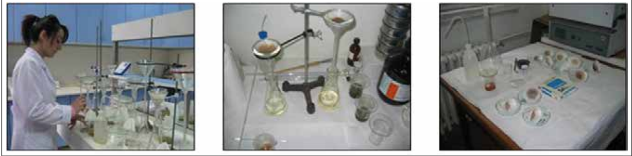
Resim 5. Asidik agrega & bağlayıcı analizi; (a) Asidik işlem (%5 HCl), (b) Süzme / yıkama ve (c) Kurutma işlemleri (MAKLAB) / Acidic aggregate & binder analysis; (a) Acidic treatment (5% HCl), (b) Filtration / washing and (c) Drying processes (MAKLAB)
