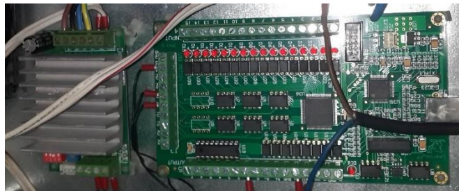
Figure 2. Mach3 CNC USB 3 Axis 200 KHz AKZ250 Leafboy77 control card.
