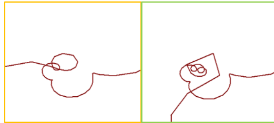
Figure. 3 Sample Images Obtained From the R-X Impedance Diagram in Mixed Transmission Lines
