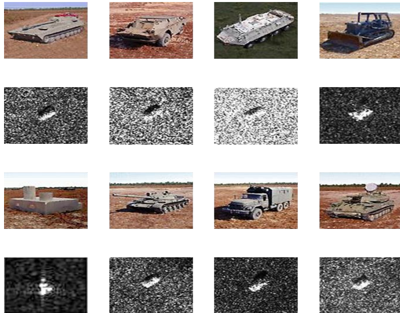
Fig. 1 The examples of 2S1, BRDM-2, BTR-60, D7, SLICY, T62, ZIL 131 and ZSU-23-4 with optical and SAR images
