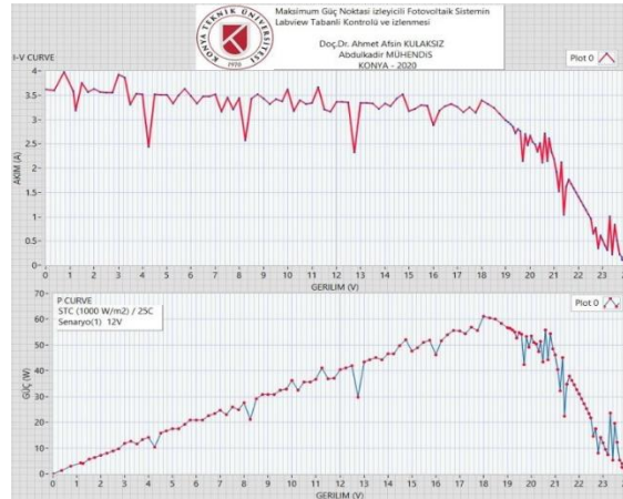
Fig. 14 The power curves of 12V battery load under (25°C, 1000 W/m 2 )
