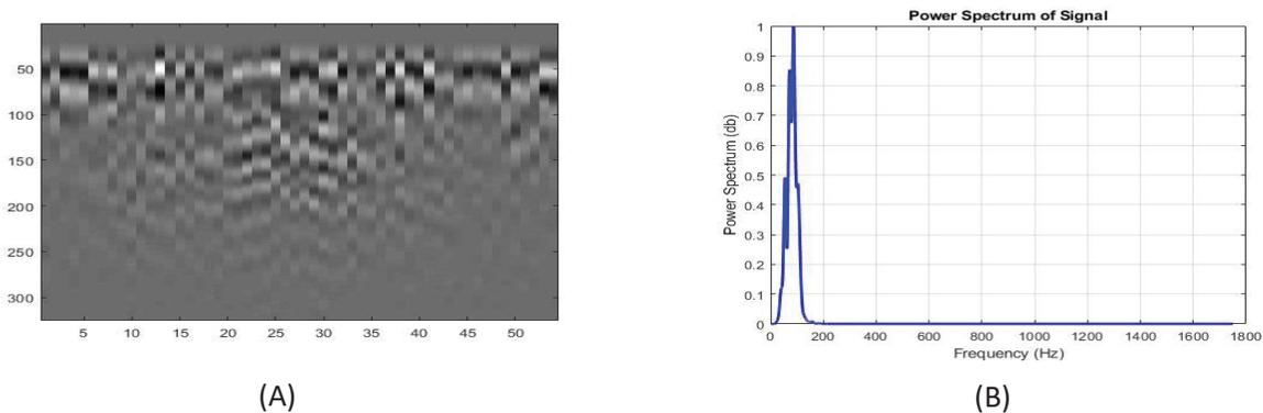
Figure 4: (A) Decluttering soil and fresh water image using MS (B) The power spectrum
