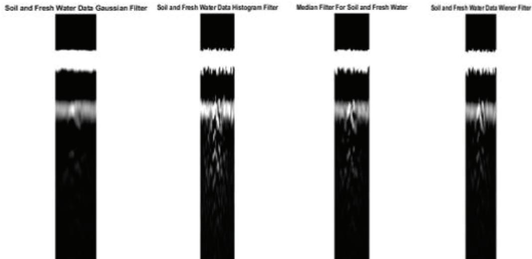
Figure 9: shows the effect of filtering over the soil and fresh water image.
