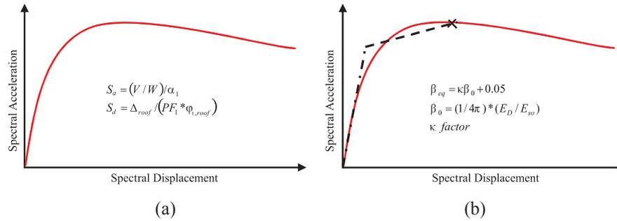
Figure 13: (a) Constructing capacity spectrum (b) Estimation of equivalent viscous damping
