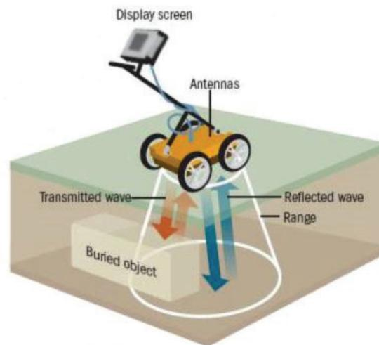
Figure 1: shows basic principle of GPR.
