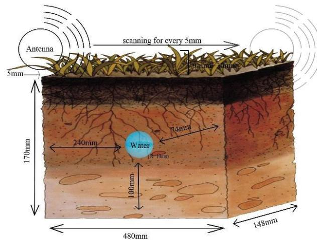
Figure 2: The geometric structure of the box.
