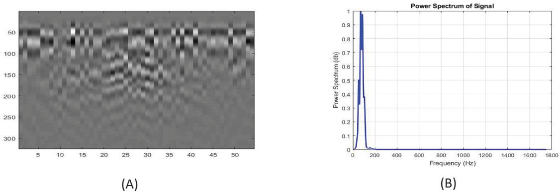
Figure 5: (A) Decluttering soil and fresh water image using SVD (B) The power spectrum.
