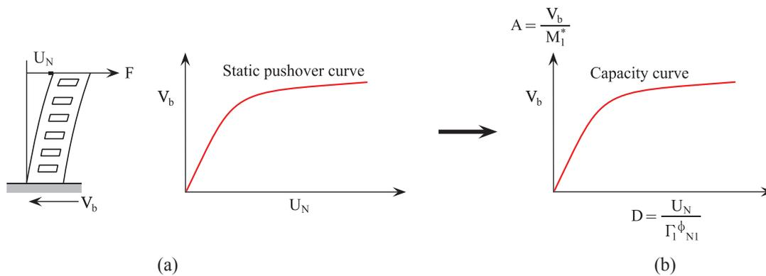
**Figure 10:** (a) Formation of the pushover curve (b) Converting the pushover curve into a capacity curve
