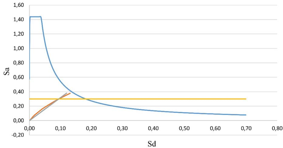
Figure 17: Spectral acceleration and spectral displacement curve
