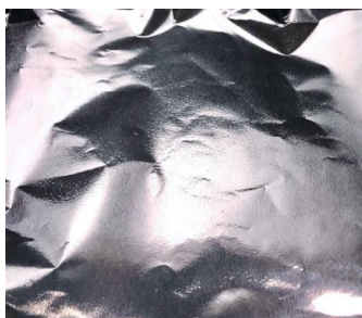
Figure 7. Picture of wet deposition on aluminum foil after electrospinning of the solution of 8 wt% PVP in DMSO at a voltage of 15 kV, a flow rate of 0.75 mL/h and a tip-to-collector of 15 cm.
