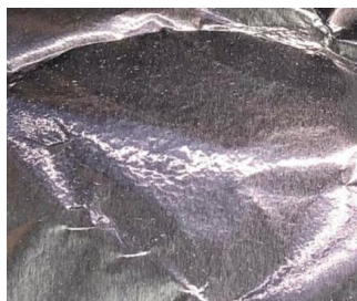
Figure 9. Picture of wet deposition on aluminum foil after electrospinning of the solution of 8 wt% PVP in DMSO/ethanol binary solvent system.
