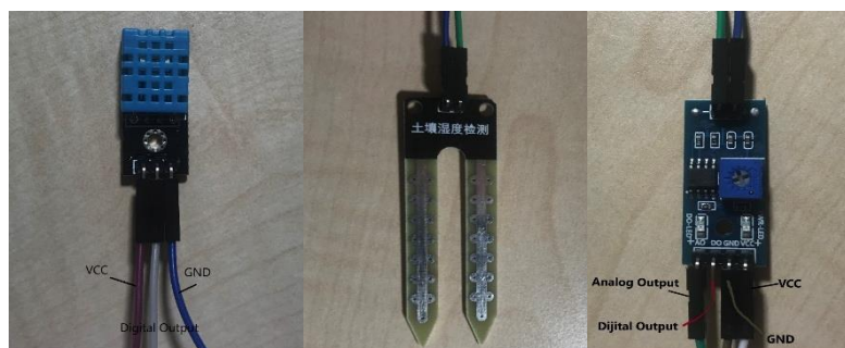
Figure 7. DHT11 with pins, Soil moisture module is placed in the soil, Soil Moisture Module main part
