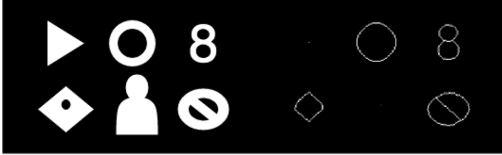
Figure 3. Shrinking behaviors of connected and non-connected objects, the original shapes are given on the left and the shrunk objects are on the right figure.
