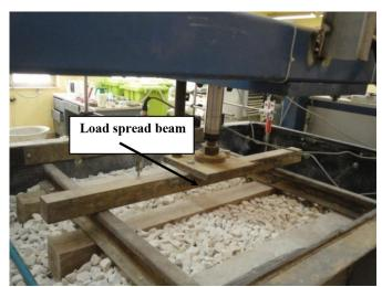
Figure 7. Load spreader beam.
