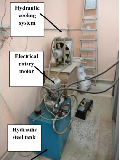
Figure 5. Hydraulic loading system.
