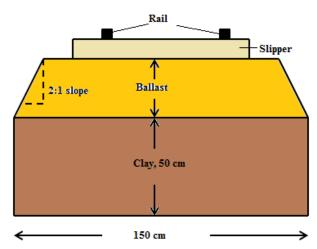
Figure 9. The laboratory test section.
