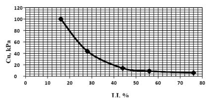
**Figure 8.** Variation of the undrained shear strength with liquidity index at 3 day curing.
