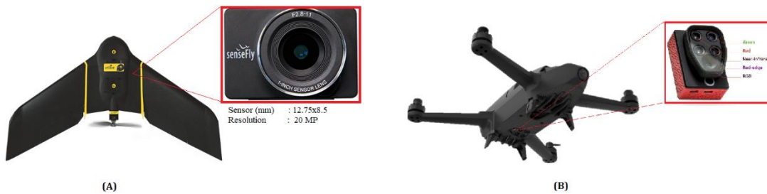
Figure 2. UAV (A: Sensefly Ebee Plus UAV and S.O.D.A Camera B: Parrot Bluegrass UAV and Parrot Sequoia+ Camera)
